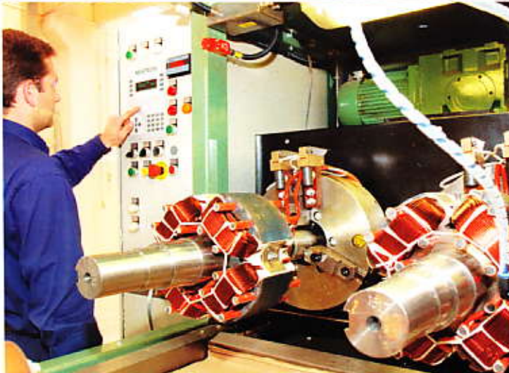
Impregnación "Dip and Roll" - "Dip and Roll" impregnation
